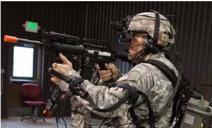
Coalescence, a wearable mixed reality defense training for air, land and sea domains, can literally merge the trainee's real world view with a synthetic environment providing a seamlessly enhanced, mixed reality. This mixed reality provides trainees with immersive and engaging training scenarios for faster learning transfer and more effective training
